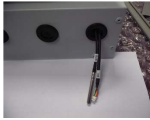
Figure 3-22 ST3 Through Bottom of Controller Box
