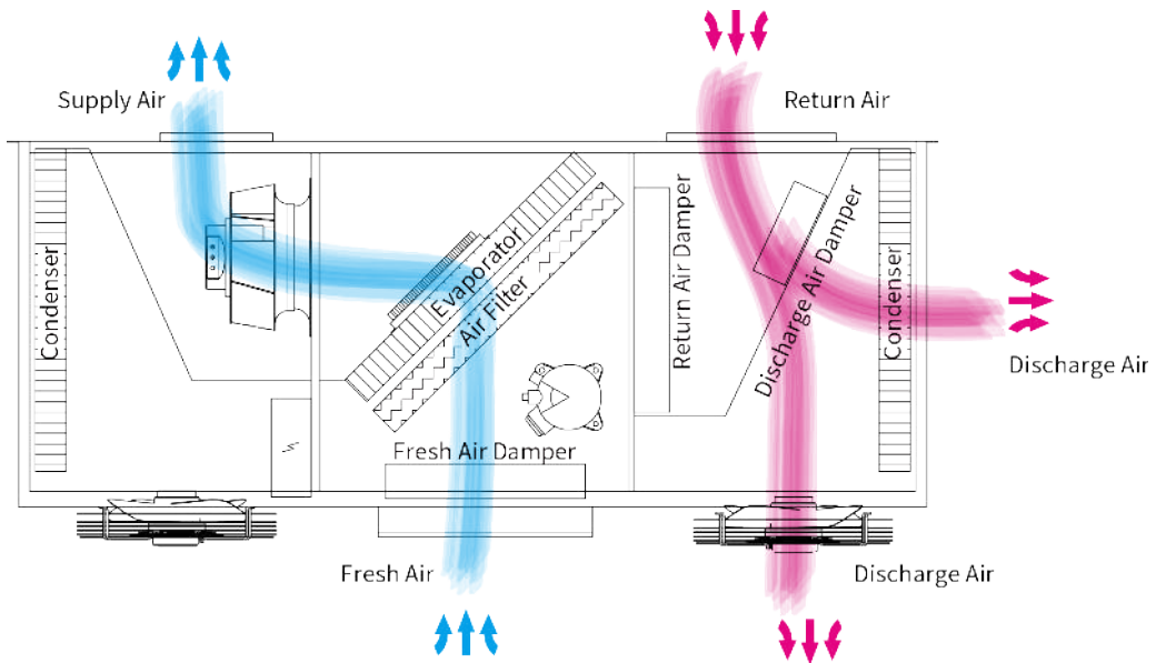
Figure 2-1 Mechanical Cooling Mode-Diagram Shown as Right Supply
