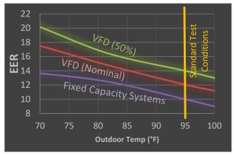
and stress and noise from the compressor will be reduced to one fourth. Redundancy is unaffected since if one unit has a mechanical cooling failure the other unit will ramp back to full capacity to maintain site temperature. This mode allows any building with redundant units to perpetually achieve 14-16 EER except during emergency situations.
