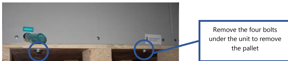
Figure 9: Remove Wooden Pallet
