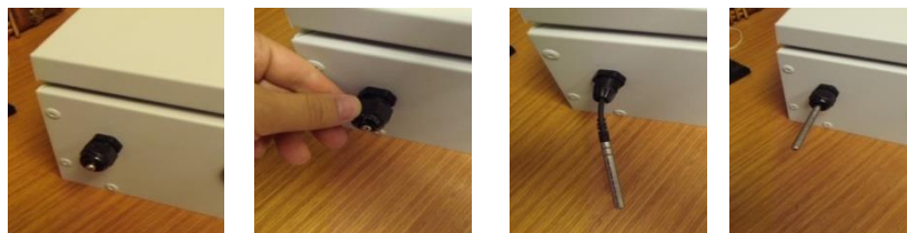
Figure 15: Position the Indoor Temperature Sensor
